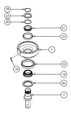
1) Remove the shaft retaining ring (18). Remove the spacer (27) and shim(s) (26).
