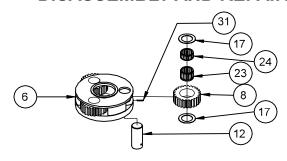
Follow the same procedure as that for the primary planetary assembly. Substitute items as indicated: planet gears (8), planet bearings (23 & 24), planet shafts (12), roll pins (31), carrier (6) and washers (17).
