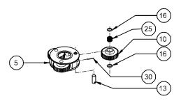
Rotate planet gears (10) to check for abnormal noise or roughness in bearings (25) or planet shafts (13). If further inspection or replacement is required, proceed as follows.
